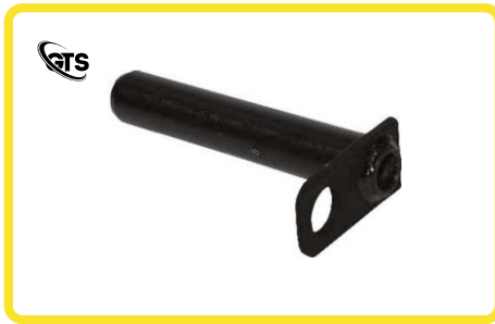
ITEM NAME LINKAGE PIN / BUCKET PIN MATERIAL EN - D SIZE 30 X 165 WITH RECTANGULAR PLATE WELDED TREATMENT & FINISH INDUCTION HARDENED & BLACK ZN. PLATED
