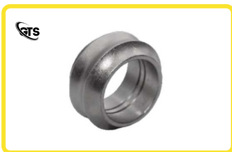
ITEM NAME SMALL PULLEY MATERIAL L.C / EN - 8 SIZE OD 50 X 28 X 35 BEARING BORE (2 NOS.) TREATMENT & FINISH WHITE ZN. PLATED
