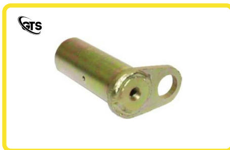
ITEM NAME LINKAGE PIN / BUCKET PIN MATERIAL EN - 8 SIZE 35 X 90 WITH ELLIPTICAL PROFILE PLATE WELDED TREATMENT & FINISH INDUCTION HARDENED & GOLDEN PLATED
