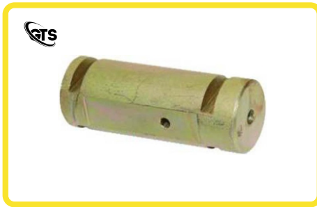
ITEM NAME CLEVIS PIN MATERIAL EN - 8 SIZE 45 X 125 TREATMENT & FINISH ZN PLATING & GOLDEN PASSIVATION
