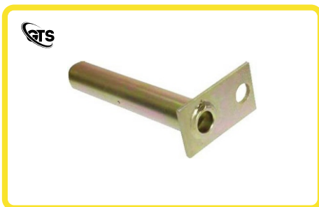
ITEM NAME LINKAGE PIN / BUCKET PIN MATERIAL EN - 8 SIZE 40 X 235 WITH RECTANGULAR PLATE WELDED TREATMENT & FINISH INDUCTION HARDENED & GOLDEN PLATED
