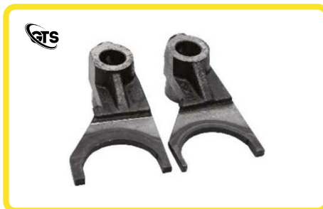
ITEM NAME FORK HD L & R SET MATERIAL EN8 - D FORGED SIZE BORE 22 X CD 106 TREATMENT & FINISH PADS INDUCTION HARDENED
