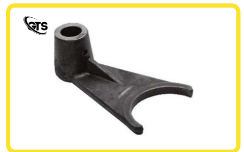
ITEM NAME FORK GDR MATERIAL EN8 - D FORGED SIZE BORE 18 X CD 106 TREATMENT & FINISH PADS INDUCTION HARDENED
