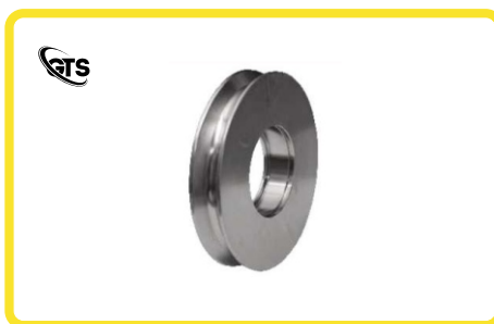
ITEM NAME PULLEY MATERIAL L.C / EN - 8 SIZE 157 X 28 TH. X 72 BEARING BORE TREATMENT & FINISH WHITE ZN. PLATED
