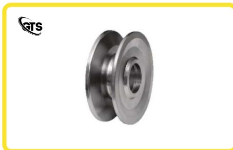
ITEM NAME DEEP GROVE PULLEY MATERIAL L.C / EN - 8 SIZE 150 X 40 38 BEARING BORE 47° TREATMENT & FINISH WHITE ZN. PLATED
