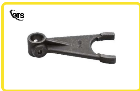
ITEM NAME FORK MATERIAL EN - 8D INVESTMENT CASTING SIZE BORE 15.80 X 89 TREATMENT & FINISH PADS INDUCTION HARDENED
