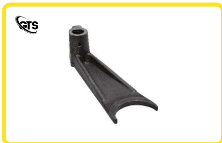
ITEM NAME FORK LONG MATERIAL EN8 - D FORGED SIZE BORE 18 X CD 180 TREATMENT & FINISH PADS INDUCTION HARDENED
