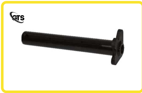
ITEM NAME LINKAGE PIN / BUCKET PIN MATERIAL EN8 - D SIZE 40 X 285 WITH PROFILE PLATE WELDED TREATMENT & FINISH INDUCTION HARDENED & BLACK ZN. PLATED
