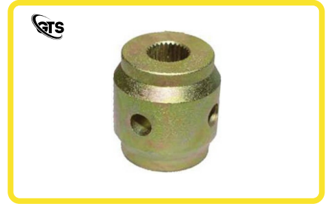
ITEM NAME BROACHED BUSH MATERIAL EN8 - D SIZE BORE 29 X 28 SPLINES TREATMENT & FINISH ZINC PLATING, GOLDEN PASSIVATION
