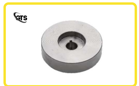
ITEM NAME BLANK PUMP GEAR MATERIAL 20MNCRS SIZE TAPER BORE 17X3° 34' 35" WITH 3MM KEYWAY BROACH TREATMENT & FINISH WHITE ZN. PLATED
