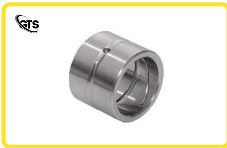
ITEM NAME BUSH WITH OIL GROOVES MATERIAL EN - 8D SIZE 40 X 50 X 40 TREATMENT & FINISH WHITE ZN. PLATED
