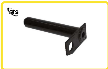
ITEM NAME LINKAGE PIN / BUCKET PIN MATERIAL EN - 8 SIZE 45 X 265 WITH ELLIPTICAL PROFILE PLATE WELDED TREATMENT & FINISH INDUCTION HARDENED & BLACK ZN. PLATED
